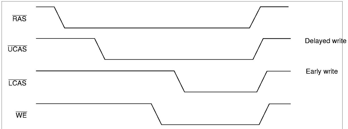
3. Closely separated upper/lower byte control is not allowed. However when the condition ( $t_{CP} \leq t_{UL}$ ) is satisfied, fast page mode can be performed.
