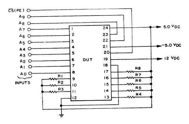
NOTES: 1. R1 thru R8 = 3.6 k $\Omega$  ±5.0% when  $\overline{\text{CS}}(\text{PE})$  input is pulsed:
