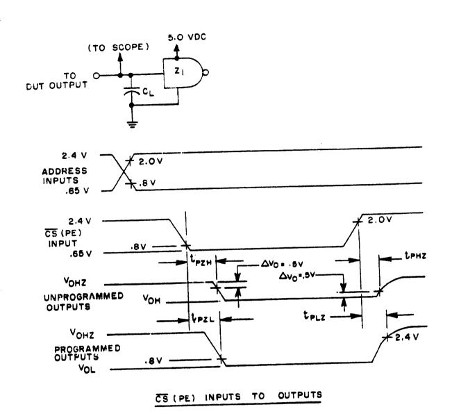
NOTES: 1.  $C_L = 100$  pF and includes jig and probe capacitance. 2.  $Z_1 = 5400$  TTL gate or equivalent.
