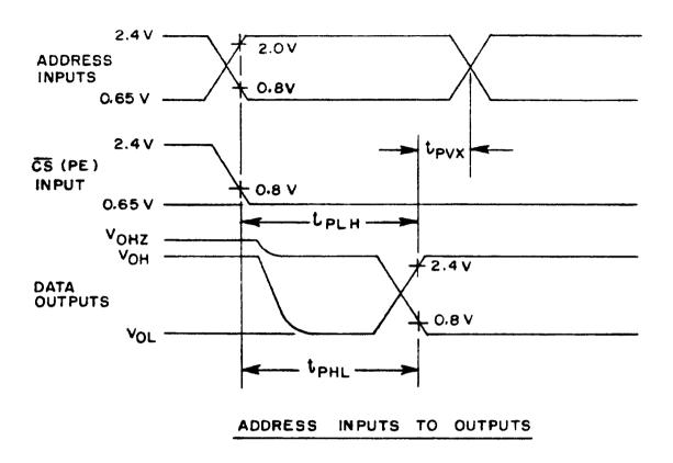
FIGURE 4. Propagation delay time test circuit and waveforms - Continued.
