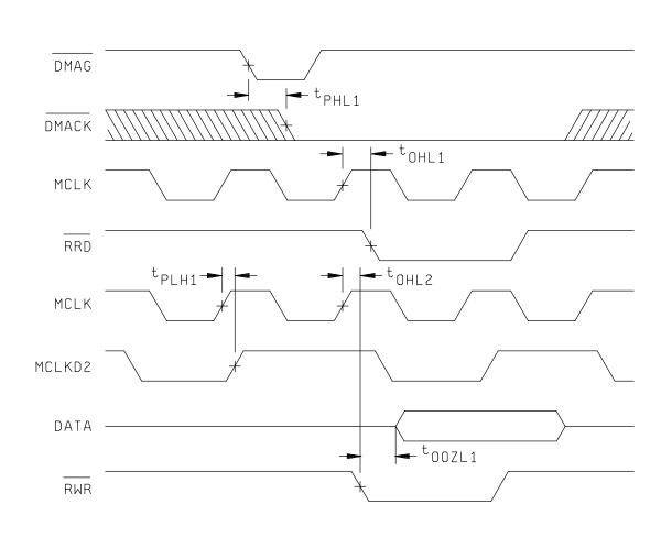
FIGURE 3. Switching test circuit and waveforms. - Continued
