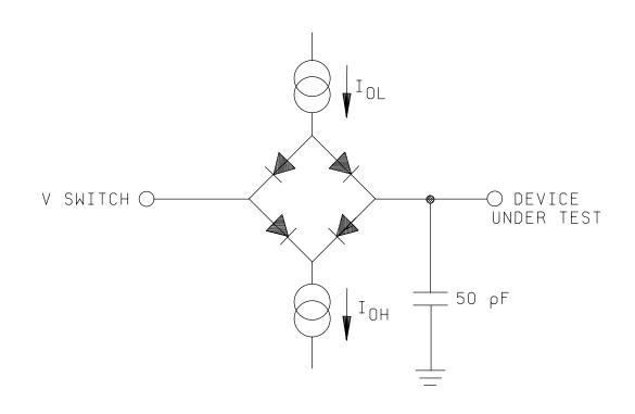
FIGURE 3. Switching test circuit and waveforms.
