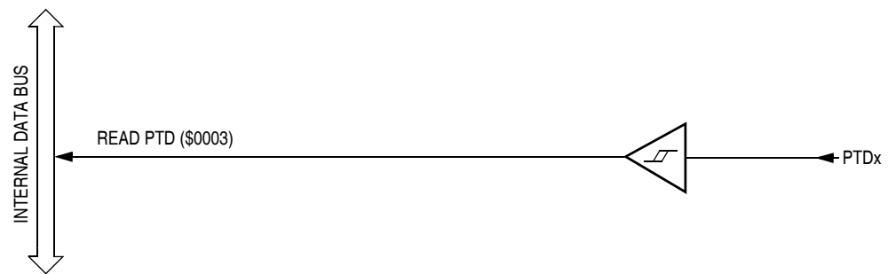
Figure 15-12. Port D Input Circuit
