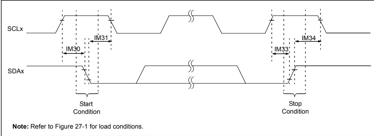
FIGURE 27-16: I2Cx BUS DATA TIMING CHARACTERISTICS (MASTER MODE)
