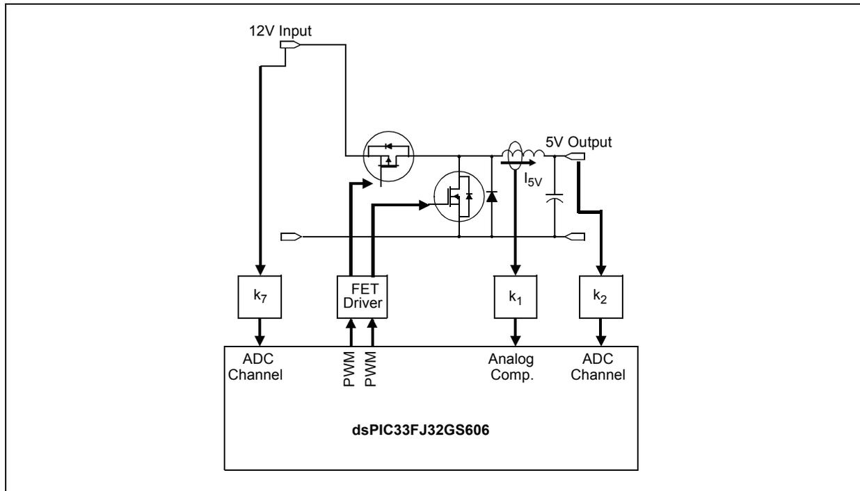
FIGURE 2-7: MULTI-PHASE SYNCHRONOUS BUCK CONVERTER
