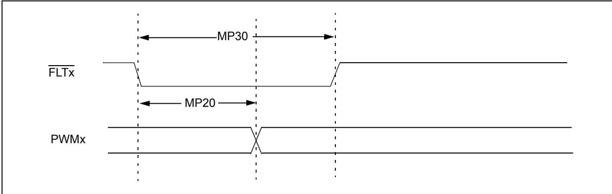
FIGURE 27-10: HIGH-SPEED PWM MODULE TIMING CHARACTERISTICS
