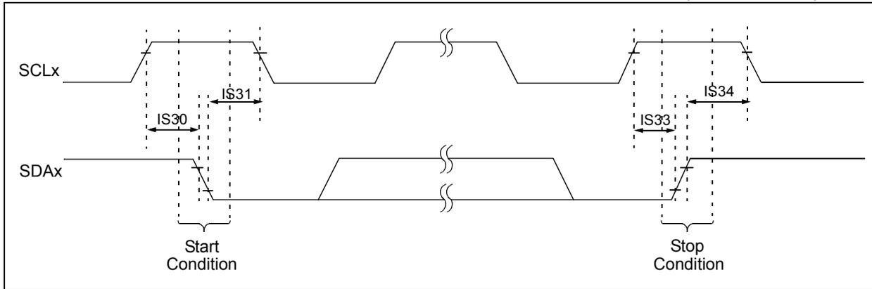
FIGURE 27-18: I2Cx BUS DATA TIMING CHARACTERISTICS (SLAVE MODE)
