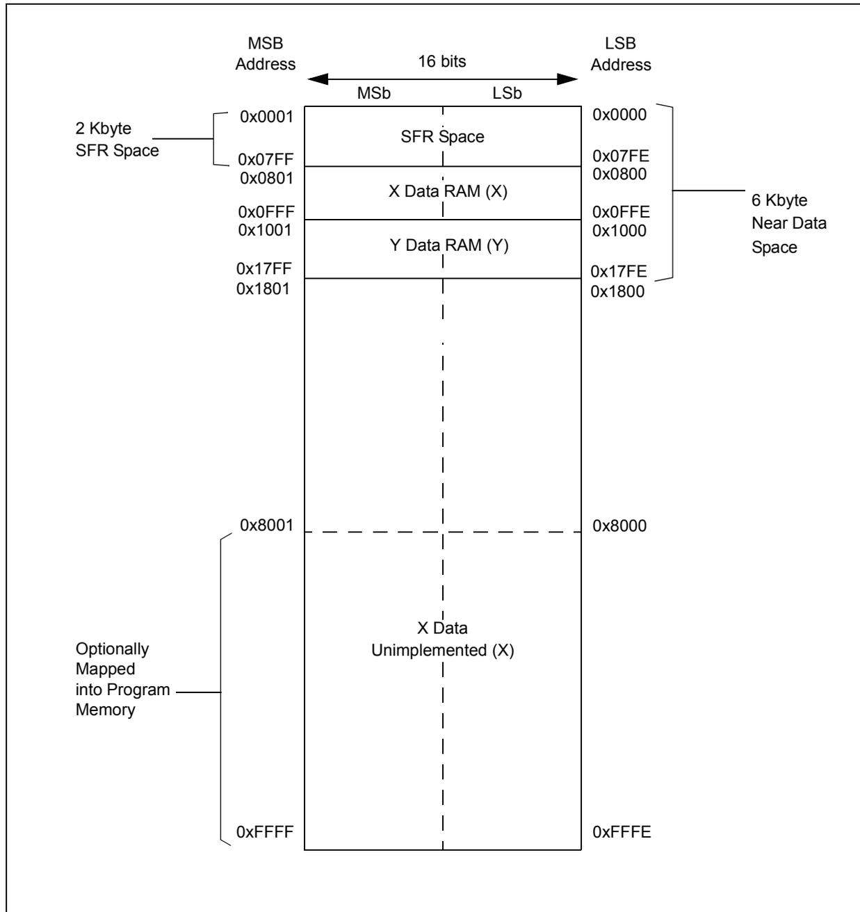
FIGURE 4-4: DATA MEMORY MAP FOR DEVICES WITH 8 KB RAM
