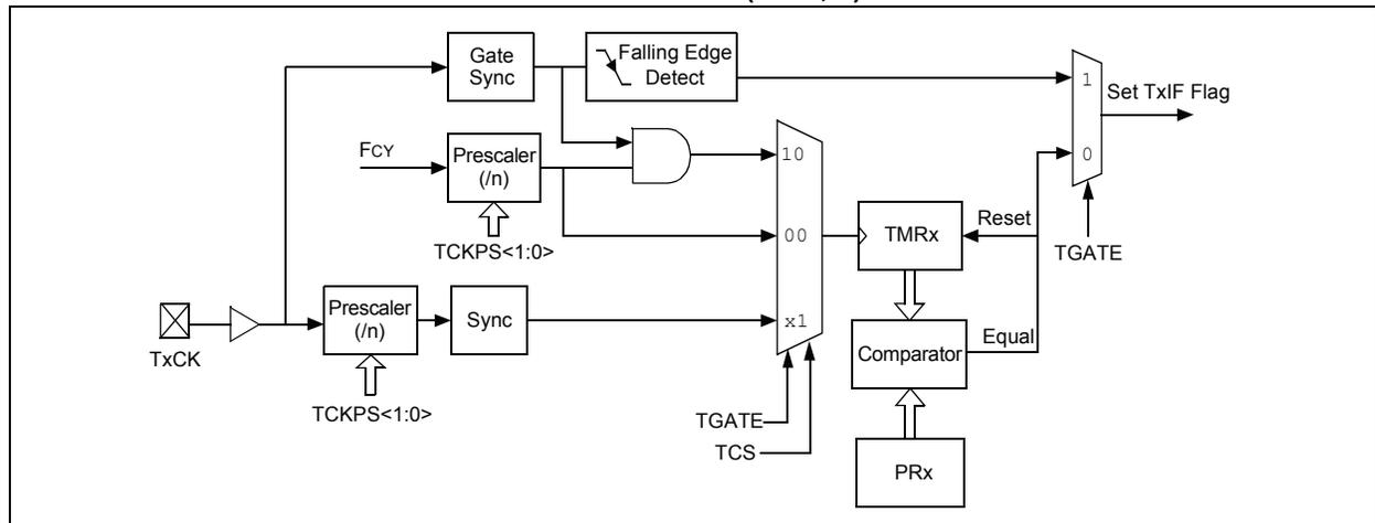
**FIGURE 13-2: TYPE C TIMER BLOCK DIAGRAM (x = 3, 5)**
