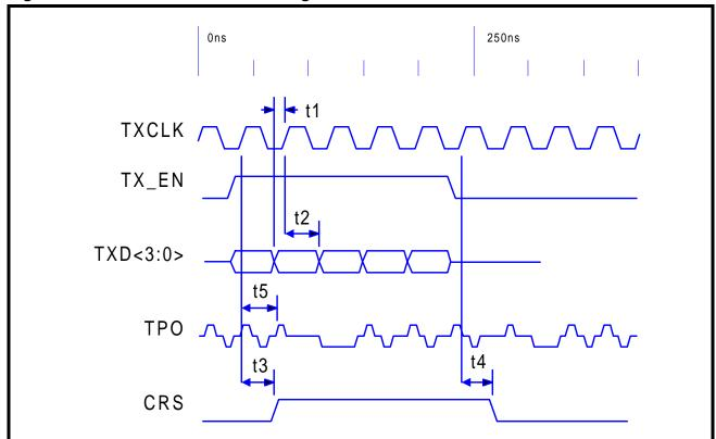
Figure 24: 100BASE-TX Transmit Timing - 4B Mode
