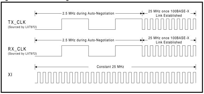
Figure 10: Link Down Clock Transition
