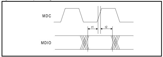
**Figure 32: MDIO Output Timing**
