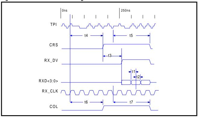
Table 25: 100BASE-TX Receive Timing Parameters - 4B Mode
