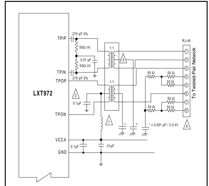
Figure 20: Typical Twisted-Pair Interface - Switch
