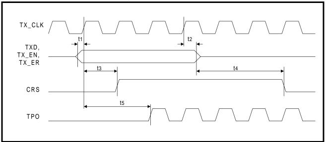
Figure 26: 10BASE-T Transmit Timing
