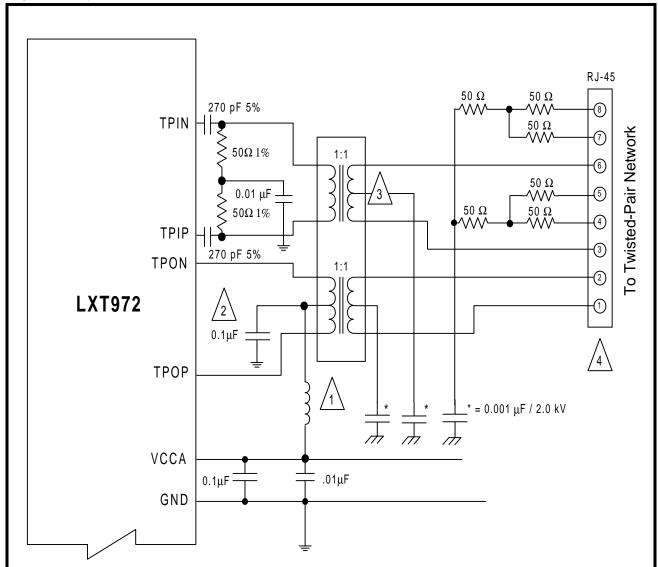
Figure 21: Typical Twisted-Pair Interface - NIC
