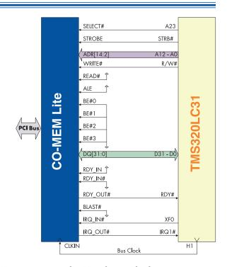
CO-MEM Lite can be configured to connect to any microprocessor. Here are two examples. Note that no glue logic is necessary.
