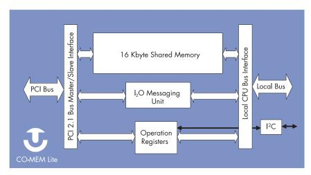
The CO-MEM Lite chip provides a simple way to interface a microprocessor to the PCI bus. The chip's internal 16-Kbyte RAM is used as a shared memory buffer between the local microprocessor and the PCI bus. An  $I_2O$  messaging unit facilitates communications between the host and local software.
