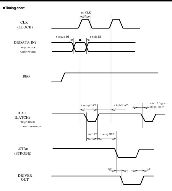
\*If delay time for Driver Out can not be secured enough, there is a possibility that VH would fluctuate greatly. Please design the circuit so that VH does not exceed peak voltage (Vp).
