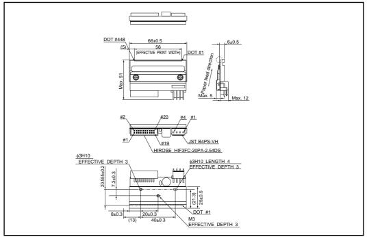
Note: No heat history control function inside the thermal printhead. External heat history control is required for high speed printing.
