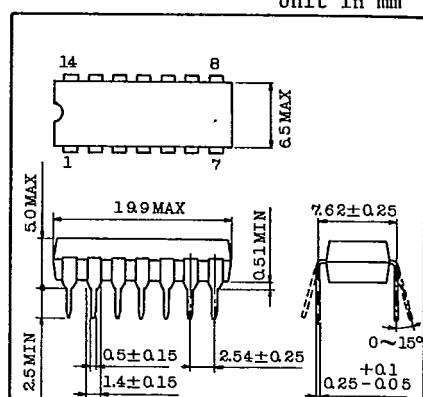
Lead pitch is 2.54 and tolerance is ±0.25 against theoretical center of each lead that is obtained on the basis of No.1 and No.14 leads.
