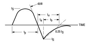
Figure 15. Diode Reverse Recovery Waveform
