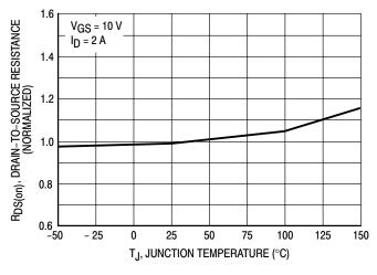
Figure 5. On–Resistance Variation with Temperature
