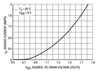
Figure 10. Diode Forward Voltage versus Current
