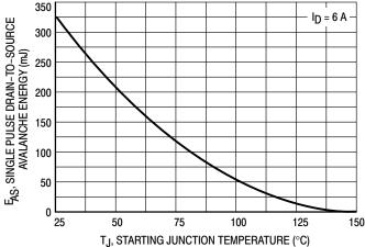
Figure 13. Maximum Avalanche Energy versus Starting Junction Temperature
