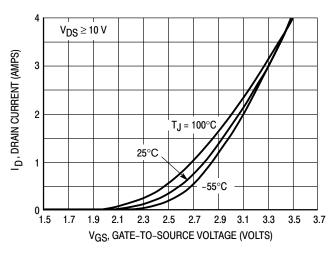
Figure 2. Transfer Characteristics
