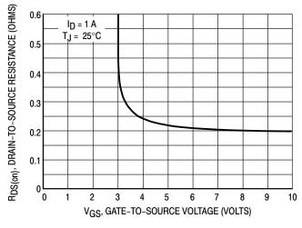
Figure 3. On–Resistance versus Gate–to–Source Voltage
