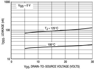
Figure 6. Drain-To-Source Leakage Current versus Voltage
