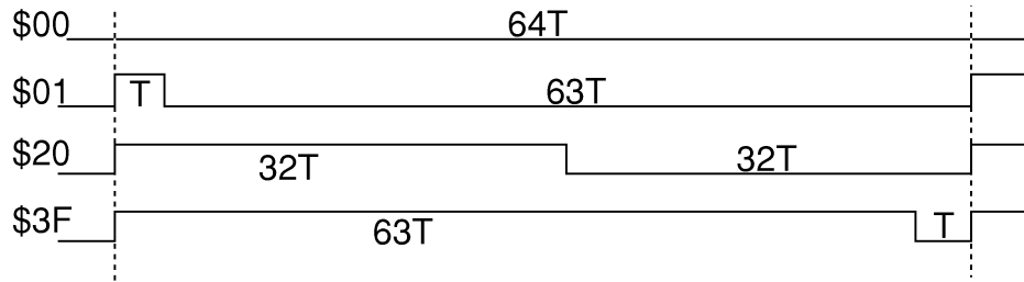
Figure 13-2. PWM Output Waveform Examples
