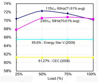
Figure 30. Measured Efficiency
