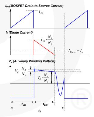
Figure 25. Key Waveforms of DCM Flyback
