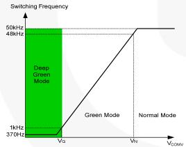
Figure 26. Switching Frequency in Green Mode
