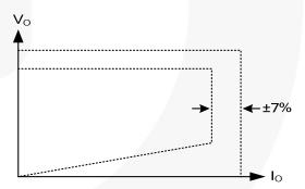
Figure 1. Typical Output V-I Characteristic
