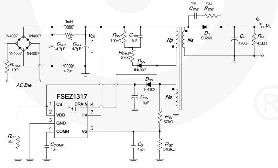
Figure 32. Schematic of Typical Application Circuit
