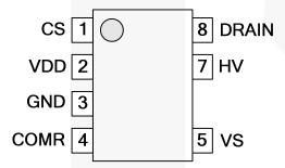
Figure 5. SOP and Dip Pin Configuration
