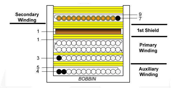
Figure 33. Transformer Specification
