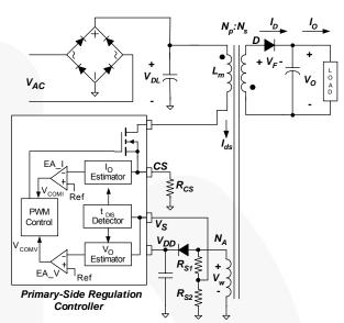
Figure 24. Simplified PSR Flyback Converter Circuit
