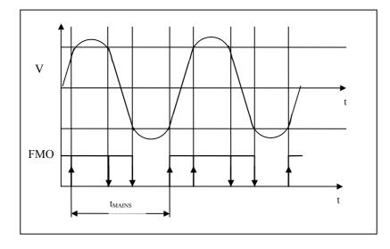
Due to comparator offset, the FMO low to high transition can be occur within a range as shown above. The time between successive low to high transitions will be equal to the mains voltage period.
