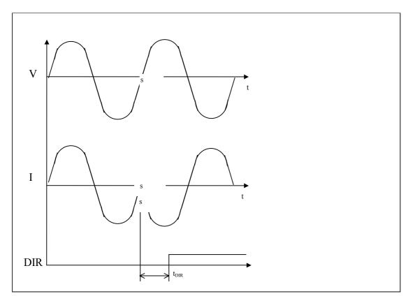
The square wave signal on FMO indicates the polarity of the mains voltage.
