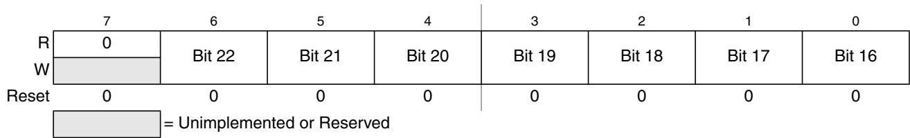
Figure 8-15. Debug Comparator Address High Register (DBGXAH)
