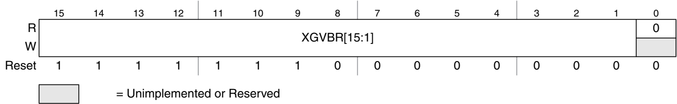
Figure 10-9. XGATE Vector Base Address Register (XGVBR)
