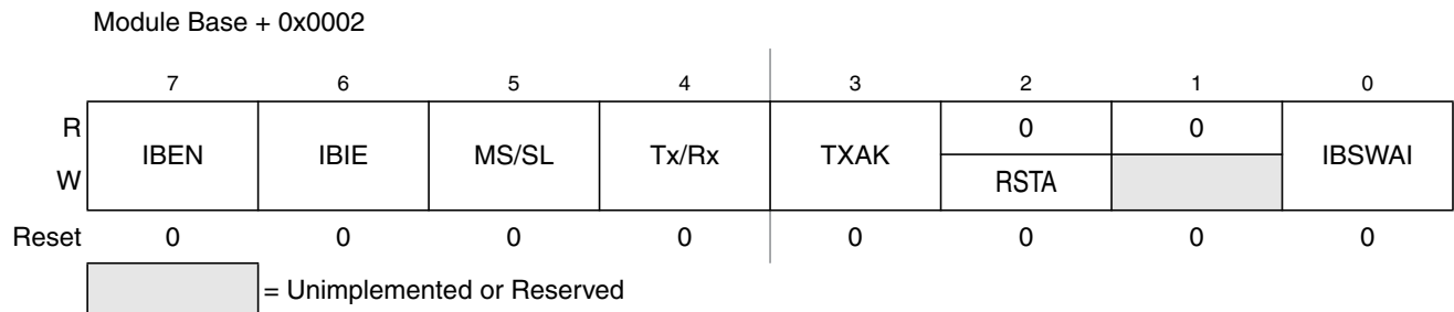
Figure 15-6. IIC Bus Control Register (IBCR)
