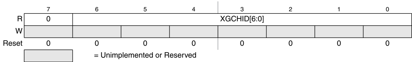
Figure 10-4. XGATE Channel ID Register (XGCHID)
