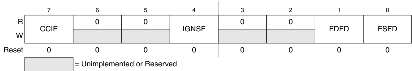
Figure 23-9. Flash Configuration Register (FCNFG)
