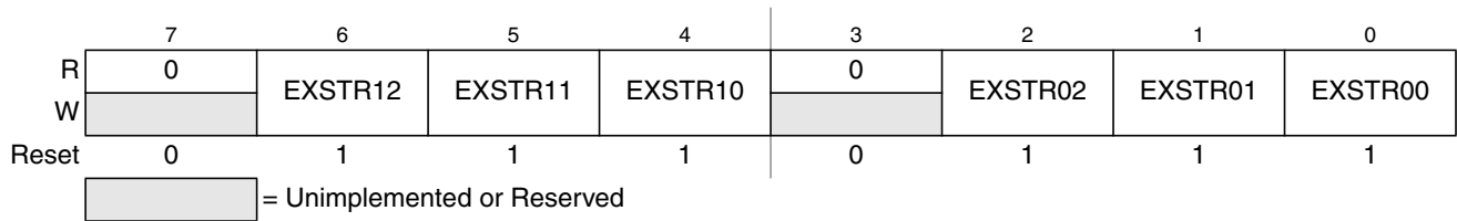
Figure 5-4. External Bus Interface Control Register 1 (EBICTL1)
