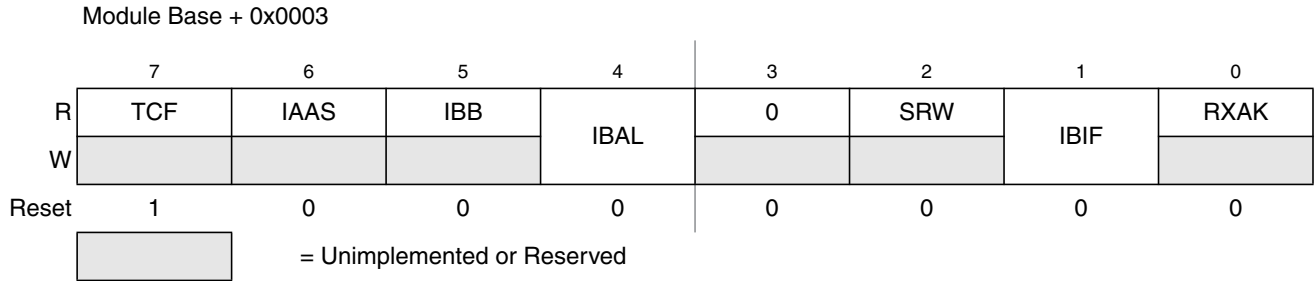
Figure 15-7. IIC Bus Status Register (IBSR)
