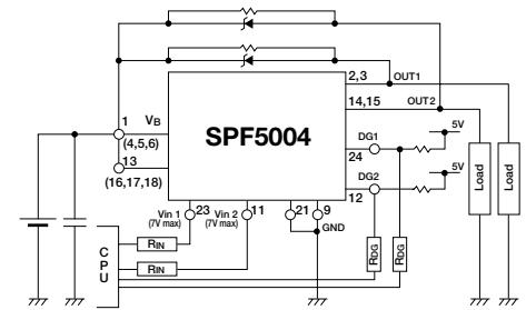
\* Make V<sub>B</sub> of 4Pin, 5Pin, 6Pin, 16Pin, 17Pin and 18Pin short from the fin to be plated by solder.
