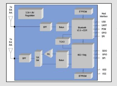
The W2CBW003 SiP delivers a complete, dual radio solution. All functionality, including the radio modem, interface control, diagnostics, timing, power regulation and coexistence are included in a certified compact ready to integrate package.
