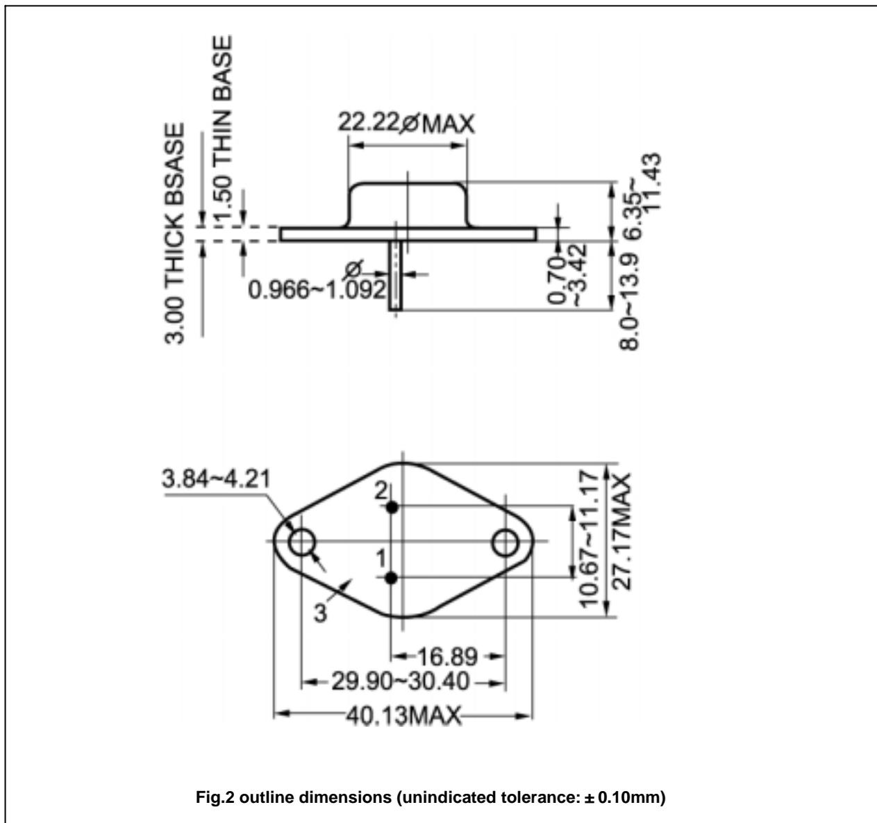
Fig.2 outline dimensions (unindicated tolerance: ± 0.10mm)
