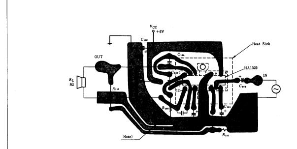
Note: The notch of ground line prevents the distortion from growing worse at flowed full-wave rectification current from the R<sub>103</sub>.
