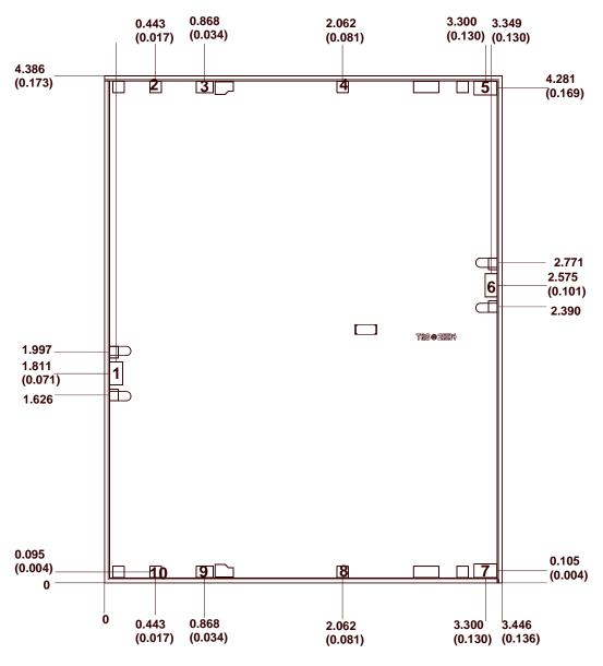
Units: millimeters (inches) Thickness: 0.100 (0.004)
