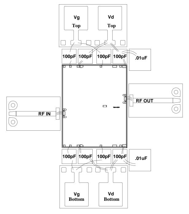
The TFNs at both RF in and RF out are flare TFNs with dimensions of 0.01 x 0.03 in on 0.01 in thick Alumina substrate.
