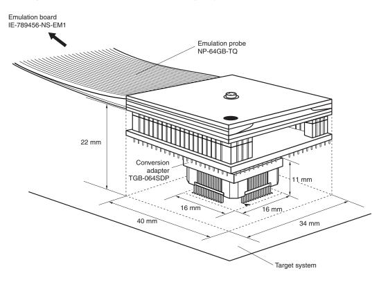
Figure B-2. Connection Conditions of Target System (When NP-64GB-TQ Is Used)
