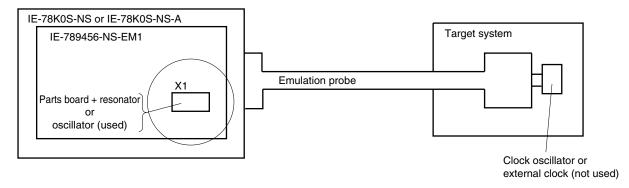
**Remark** The clock that is supplied by the resonator of the IE-789456-NS-EM1 (encircled in the figure) or the oscillator is used.
