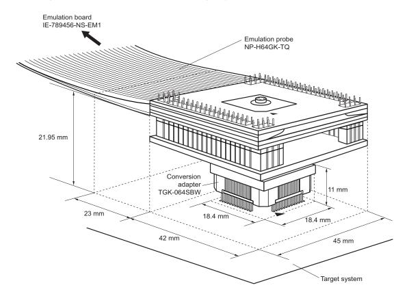
Figure B-6. Connection Conditions of Target System (When NP-H64GK-TQ Is Used)
