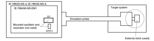
Figure 3-8. When Supplying Pulse from Target System
