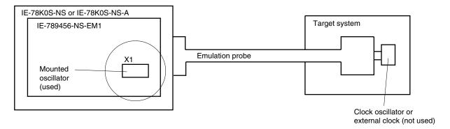
**Remark** The clock that is supplied by the oscillator of the IE-789456-NS-EM1 (encircled in the figure) is used.
