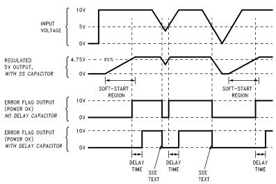
FIGURE 14. Timing Diagram for 5V Output
