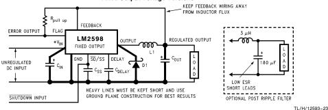
Component Values shown are for  $V_{\mbox{\footnotesize{IN}}} = 15 \mbox{\footnotesize{V}},$
