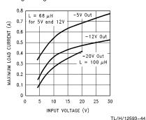
FIGURE 27. Maximum Load Current for Inverting Regulator Circuit
