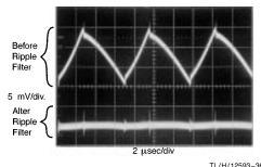
FIGURE 19. Post Ripple Filter Waveform
