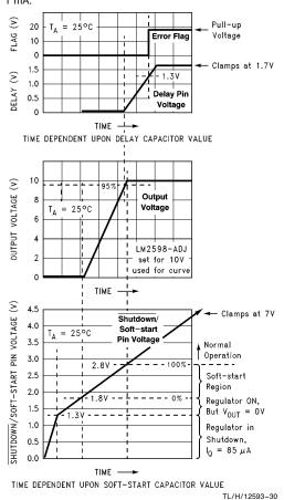
FIGURE 13. Soft-start, Delay, Error, Output
