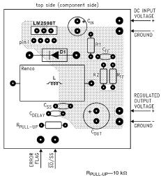
$C_{IN}$ —150  $\mu$ F/50V, Aluminum Electrolytic, Panasonic "HFQ series"  $C_{OUT}$ —120  $\mu$ F/25V Aluminum Electrolytic, Panasonic "HFQ series"
