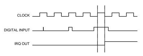
Fig. 7-1 — Digital Interrupt Timing Diagram
