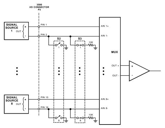
Fig. 2-2 — 3500 Input Connection Diagram
