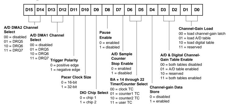
A write to BA + 2 sets up the Control Register shown above:
