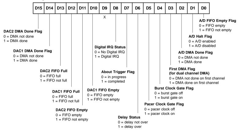
A read provides the status bits defined below. Starting with bit 0, these status bits show:
