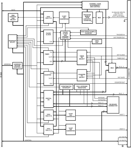
The 3500 has four major circuits, the A/D, the D/A, the timer/counters, and the digital I/O lines. Figure 3-1 shows the block diagram of the board. This chapter describes the hardware which makes up the major circuits.
