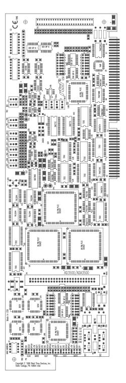
Fig. 1-1 — Board Layout Showing Factory-Configured Settings
