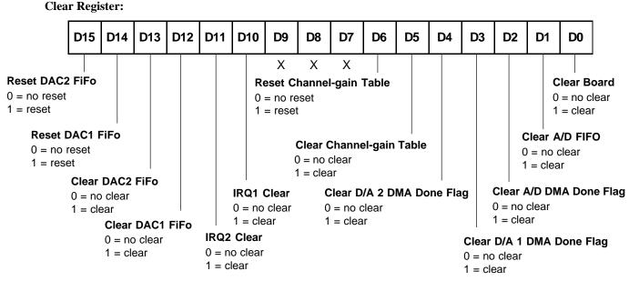
The value programmed in this register determines which clear, enable, and reset operations are carried out when a read at BA + 0 is executed. Setting a bit high clears or enables the defined operation. This register's bits are described below:
