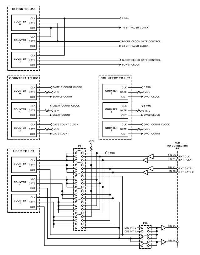
Fig. 3-2 — Timer/Counter Circuit Block Diagram
