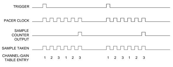
Fig. 5-9 — Timing Diagram, Programmable Multiscan
