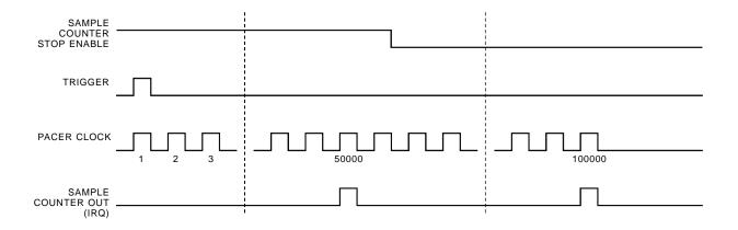
Fig. 5-12 — Timing Diagram for Cycling the Sample Counter
