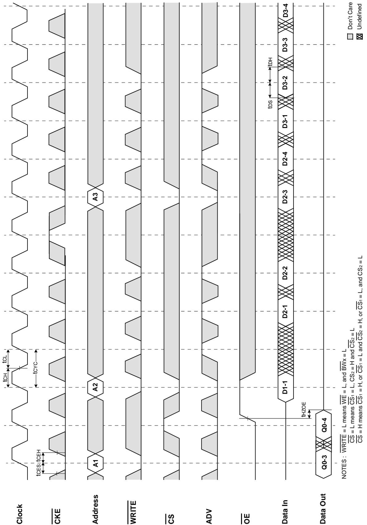
TIMING WAVEFORM OF SINGLE READ/WRITE
