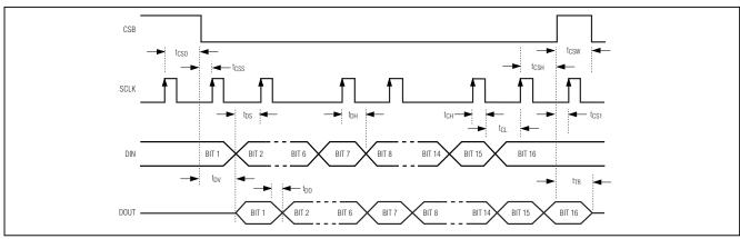
Figure 1. MAX2820/MAX2821 Serial-Interface Timing Diagram
