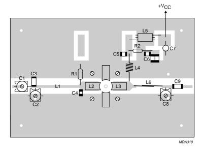
The circuit and the components are situated on one side of the P.T.F.E. fibre-glass board; the other side is unetched copper serving as a groundplane. Earth connections are made by using hollow rivets, fixing-screws and copper straps at the input and output and under the two emitters to provide a direct contact between the copper on the component side and the groundplane.
