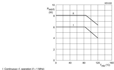
Fig.2 Power/temperature derating curves.
