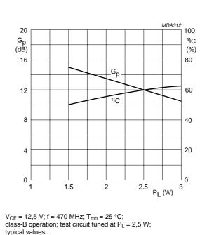
Fig.8 Power gain and efficiency versus load power.
