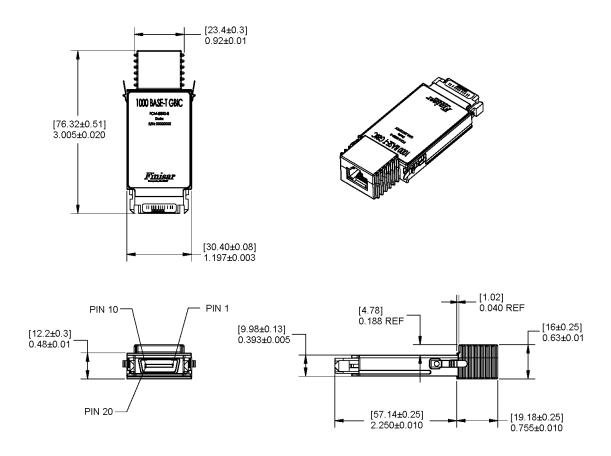
Figure 1. FCM-8520/8521-3 mechanical dimensions
