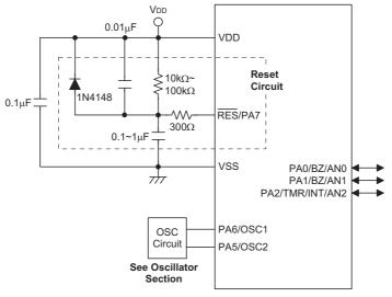
Note: "\*" The components in "Reset Circuit" The HT48R005 hasn't the AN0~AN2 pins.
