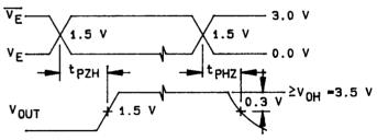
FIGURE 3. Test circuit and switching waveforms.
