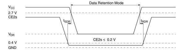
Figure 35. CE2s Controlled Data Retention Mode
