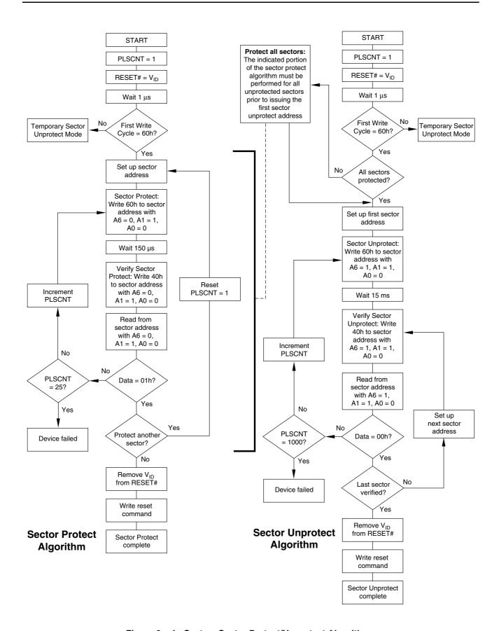
Figure 2. In-System Sector Protect/Unprotect Algorithms
