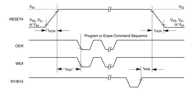
Figure 26. Temporary Sector Unprotect Timing Diagram
