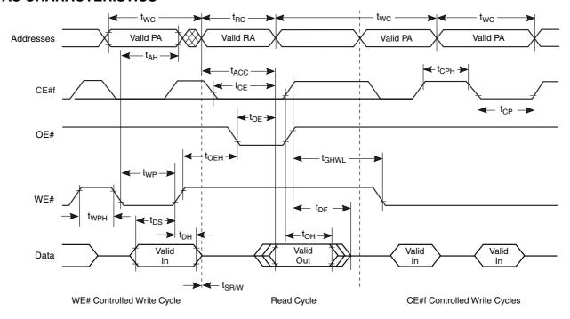
Figure 22. Back-to-back Read/Write Cycle Timings
