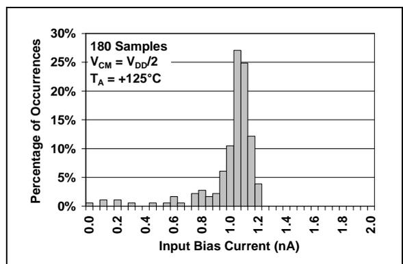
**FIGURE 2-6:** Input Bias Current at  $+125^\circ\text{C}$ .
