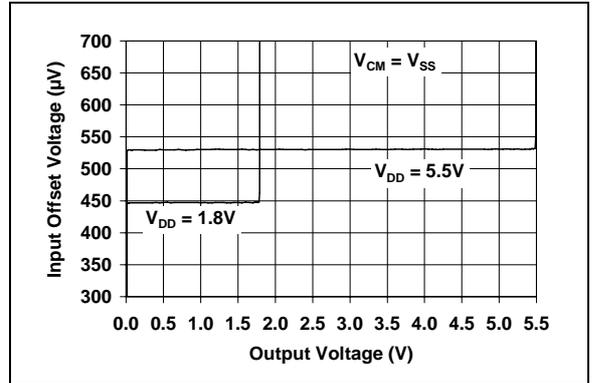
**FIGURE 2-11:** Input Offset Voltage vs. Output Voltage.
