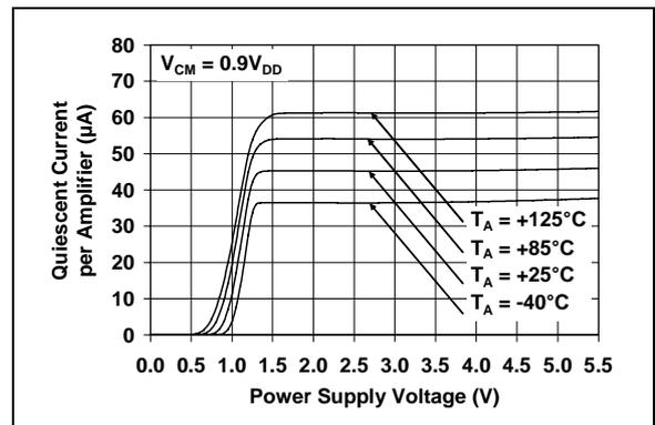
**FIGURE 2-18:** Quiescent Current vs. Power Supply Voltage.
