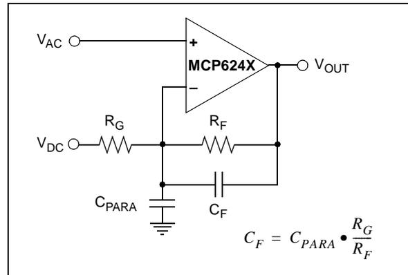
**FIGURE 4-8:** Effect of Parasitic Capacitance at the Input.
