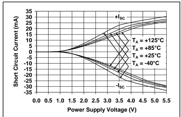
**FIGURE 2-12:** Output Short-Circuit Current vs. Ambient Temperature.
