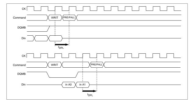
**Burst Length = 4** (To stop write operation)
