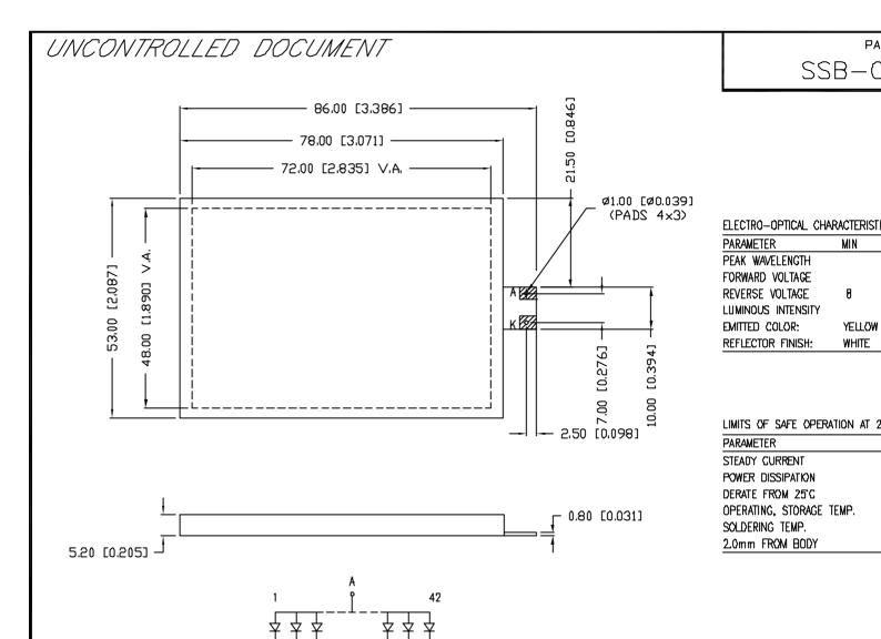
\*UNIESS OTHERWISE SPECIFIED TOLERANCES PER DECIMAL PRECISION ARE: X=±1 (±0.039), XX=±0.5 (±0.020), XXX=±0.25 (±0.010), XXXX=±0.127 (±0.005). LEAD SIZE=±0.05 (±0.0102), LEAD LENGTH=±0
