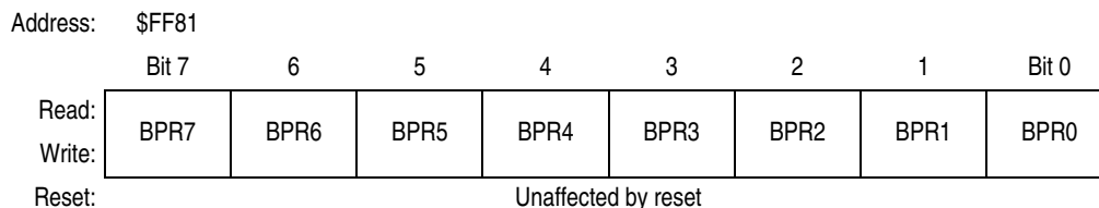
Figure 2-8. FLASH-2 Block Protect Register (FL2BPR)
