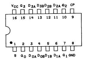
FIGURE 1. Terminal connections.
