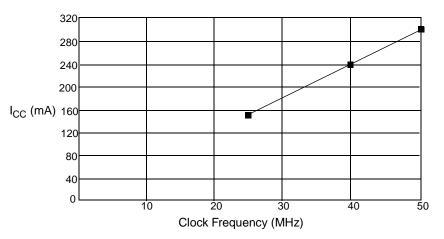
Figure 10. Typical I<sub>cc</sub> Versus Frequency
