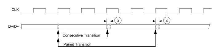
Figure 28. USB Receiver Jitter Tolerance
