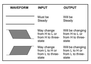
Figure 13. Key to Switching Waveforms
