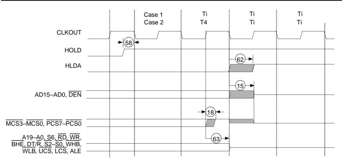
Figure 23. Entering Bus Hold Waveforms
