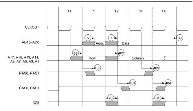
Figure 32. DRAM Write Cycle without Wait States Waveform
