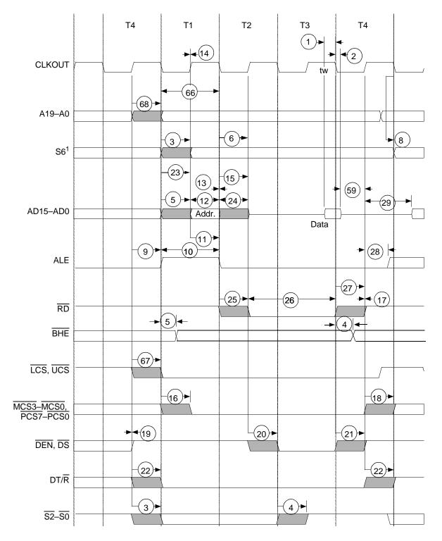
1. S6 is not valid for the first fetch until the timing for parameter 3 (status active delay ( $t_{CHSV}$ )) is met.
