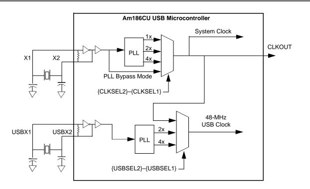
Figure 5. System and USB Clock Generation
