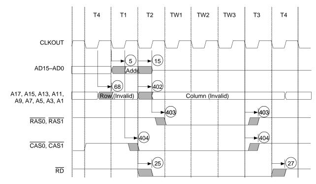
Figure 34. DRAM Refresh Cycle Waveform
