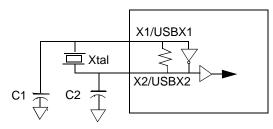
Figure 7. External Interface to Support Clocks— Fundamental Mode Crystal
