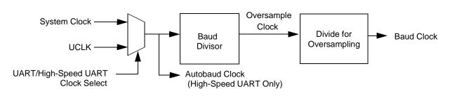
Figure 9. UART and High-Speed UART Clocks
