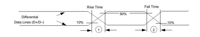
Figure 27. USB Data Signal Rise and Fall Times
