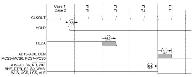
Figure 24. Exiting Bus Hold Waveforms
