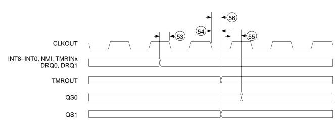
Figure 17. Peripheral Waveforms
