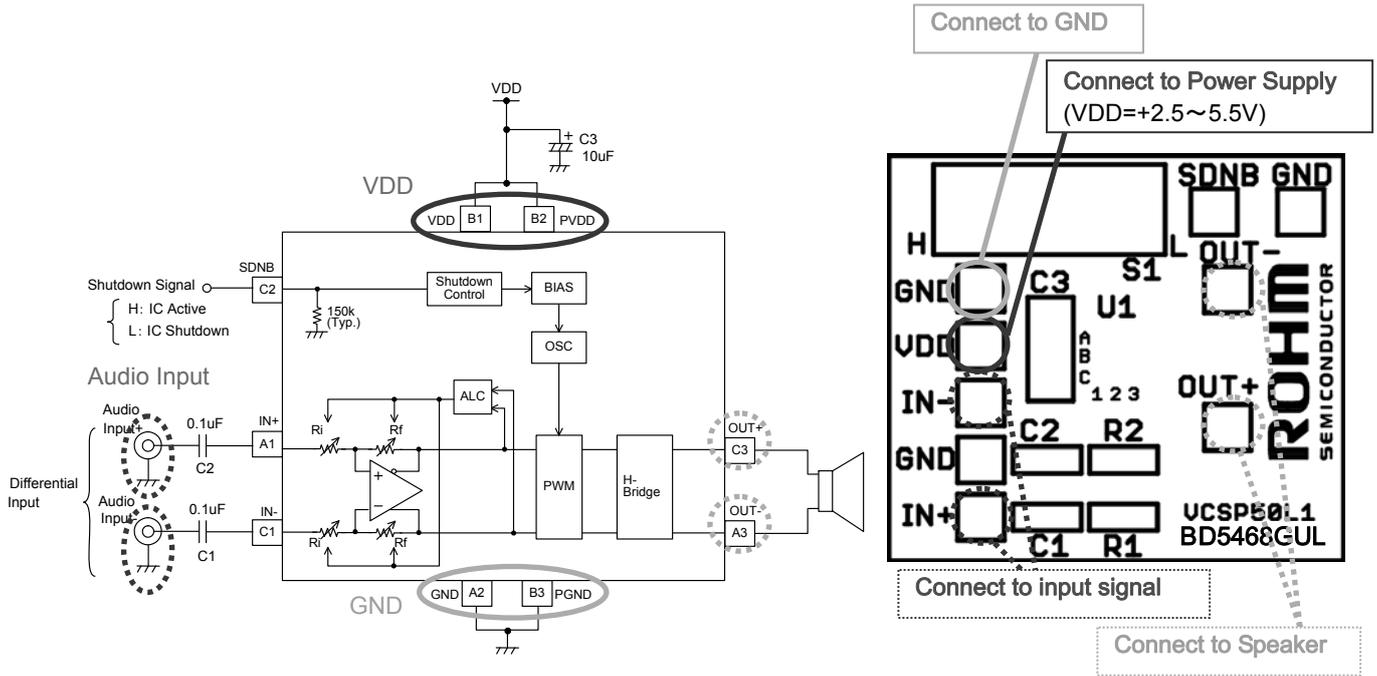
※Power Supply terminals VDD(B1), PVDD(B2) are SHORT in the board pattern and use a single power.
