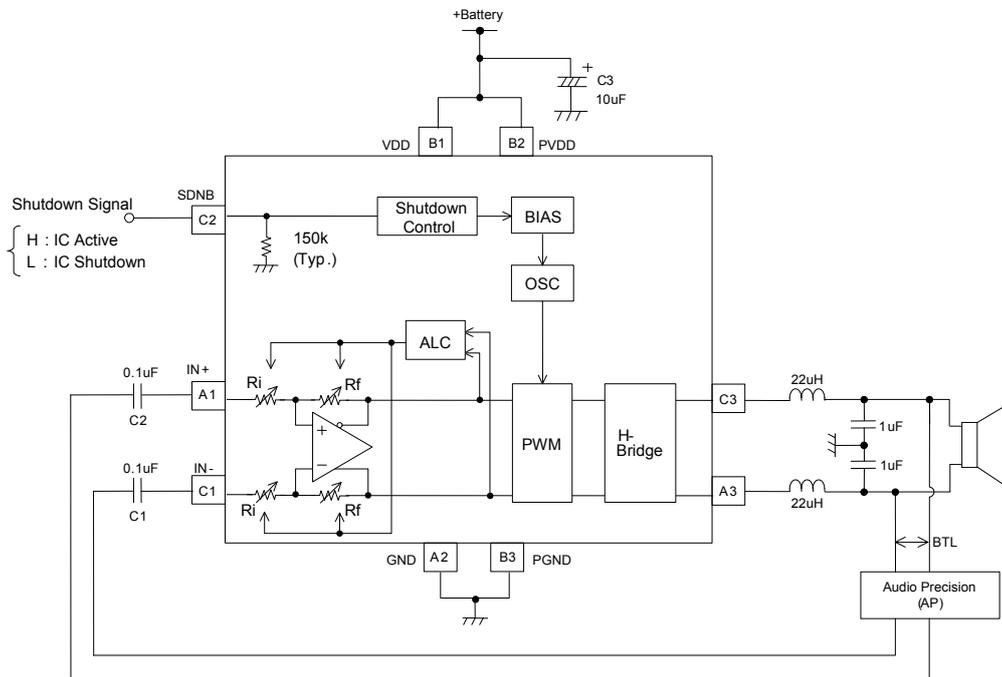
Audio characteristics can be measured to insert LC filter between output pin and speaker load, if you don't have measurement equipment for switching amplifier, like AUX-0025, Audio Precision. Arrange the LC filter directly close to output pin.
