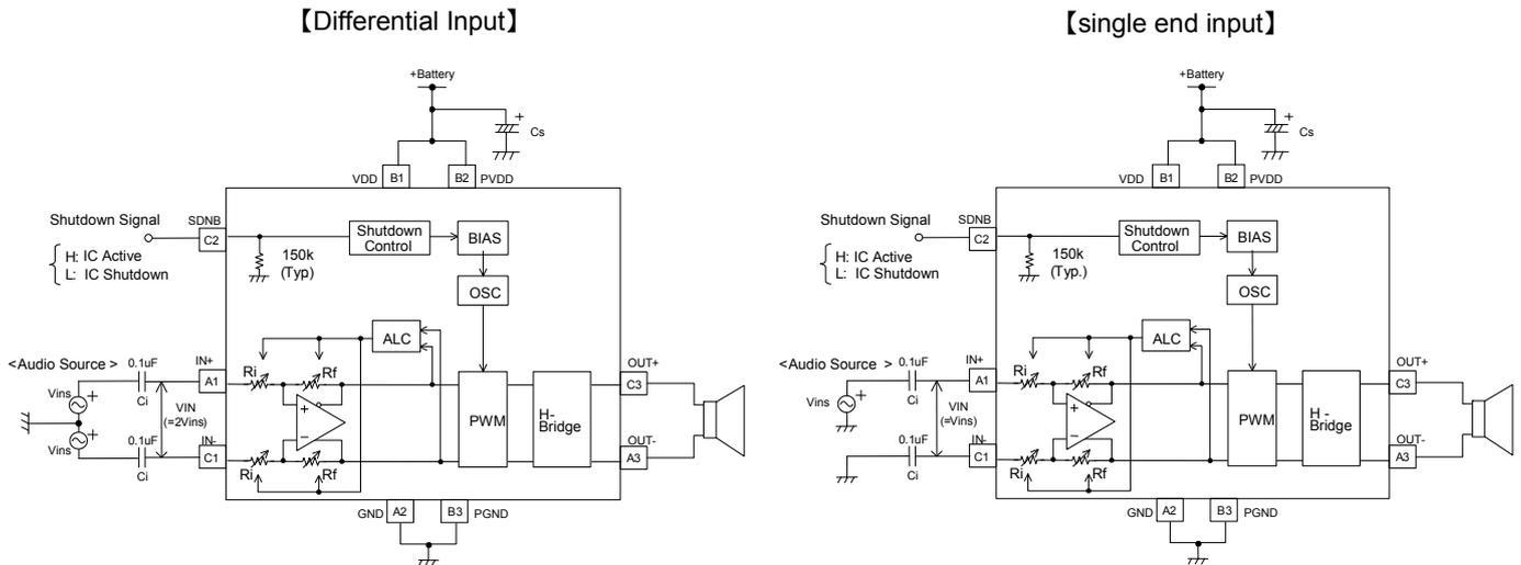
When Input Level is calculated at IC typical and audio source typical, when input coupling capacitor (Ci) value is large enough, every gain during the differential input and single end input will become:
