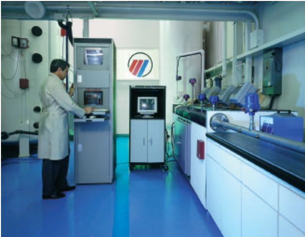
In The Magnetrol Product Calibration Lab , Thermatel products are calibrated and tested to meet customer specifications. Calibrations traceable to NIST.
