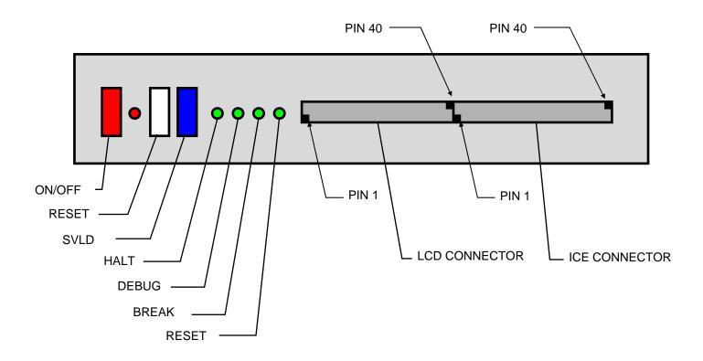
The RESET switch will perform a hardware reset to the entire emulator, however it will not reinitialise peripheral RAM or trace and program memory. It will set peripheral registers to their reset values as specified in the respective microcontroller data sheets.
