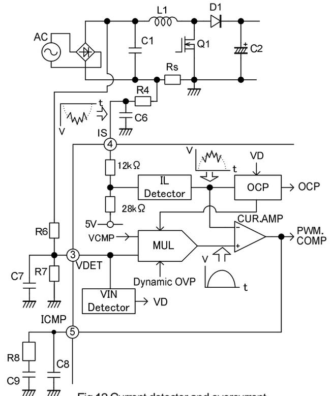
Fig.12 Current detector and overcurrent protection circuit
