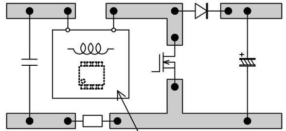
IC is arranged under inductor (or on immediately opposite side on circuit board)
