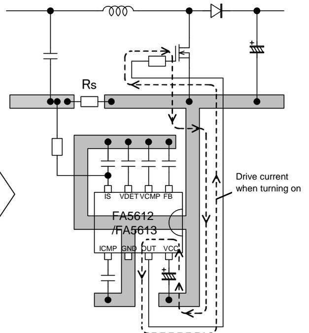
Fig.38 Example of GND wiring
