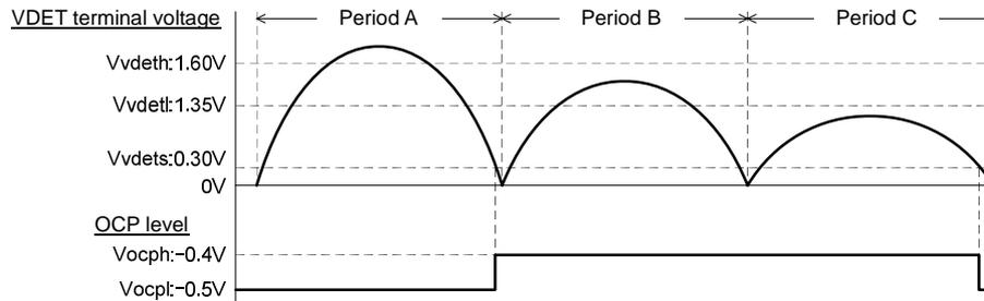
Fig.13 Overcurrent protection (OCP) level and VDET voltage
