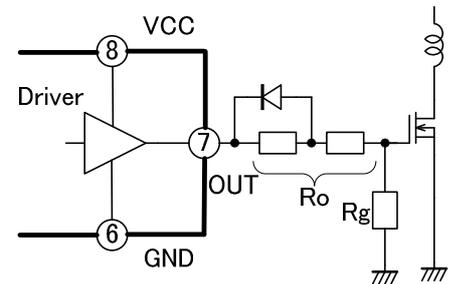
Fig.27 OUT pin circuit (2)
