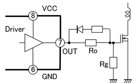
Fig.28 OUT pin circuit (3)
