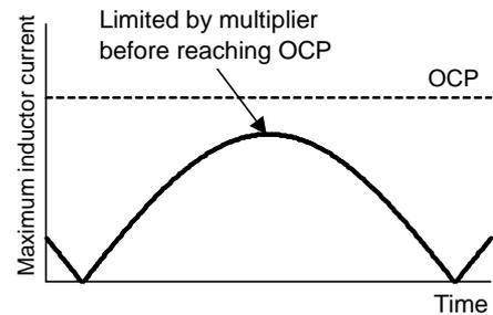
Fig.22 Maximum inductor current at low input voltage
