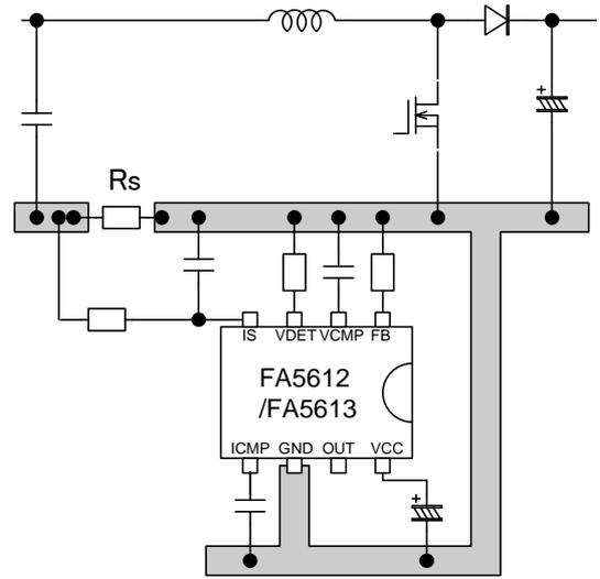
Fig.36 Example of inadvisable GND wiring
