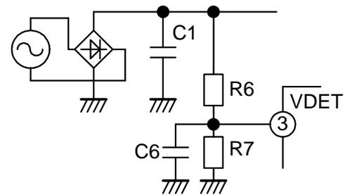
Fig.17 VDET terminal circuit
