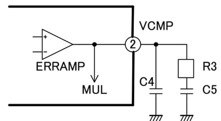
Fig.16 VCMP pin circuit
