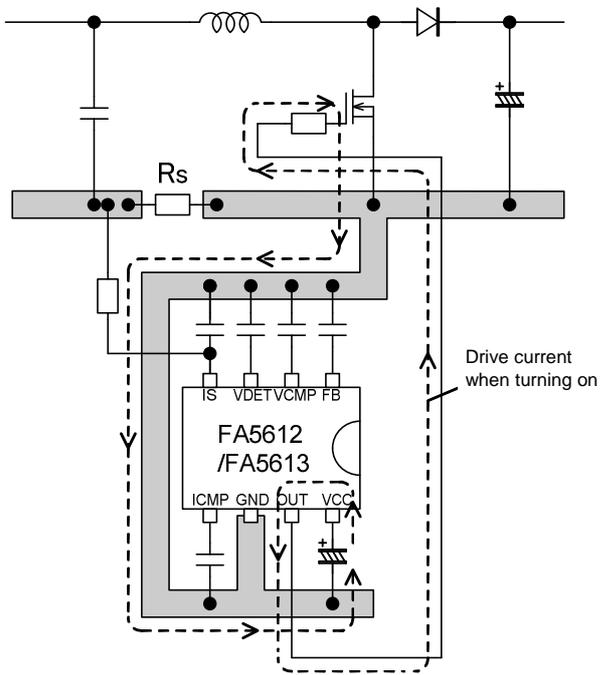
Fig.37 Example of inadvisable GND wiring
