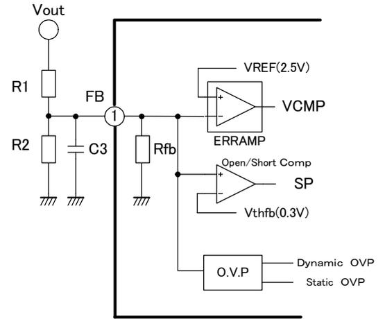
Fig.15 FB pin circuit
