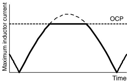
Fig.21 Maximum inductor current at high input voltage
