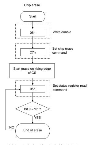
\* Automatically placed in write disabled state at the end of the erase
