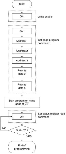
\* Automatically placed in write disabled state at the end of the programming operation.
