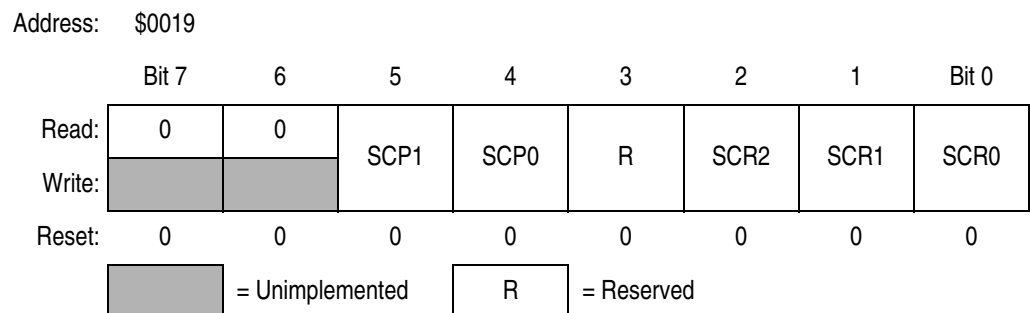
Figure 18-18. SCI Baud Rate Register (SCBR)
