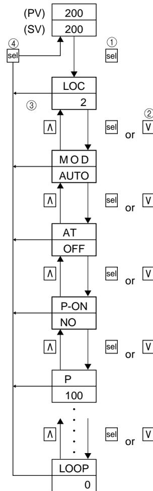
① Keep  $\text{sel}$  key pressed for about 3 sec. in PV/SV display condition.
