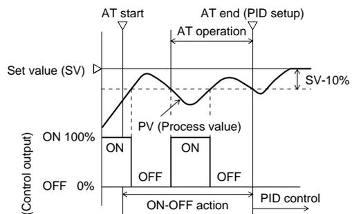
Remarks: (1) Once auto-tuning has been made, PID parameter values are retained despite power-off operation. Therefore, auto-tuning need not be repeated for the subsequent operations.
