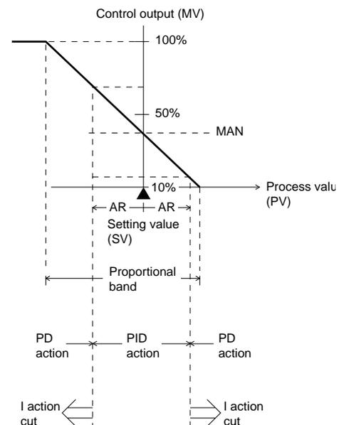
Note : \*ARW: INTEGRAL action is cut when PV is out range of AR value.
