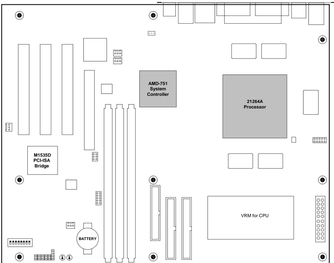
Figure 3-1 Thermally-sensitive Components
