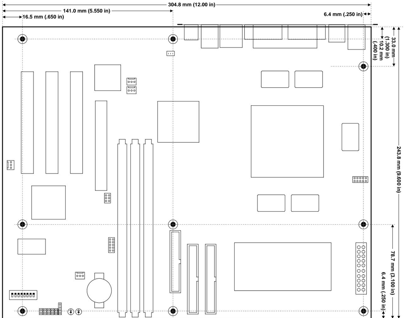
**Figure 3-2 UP1100 Mounting Hole Specification**
