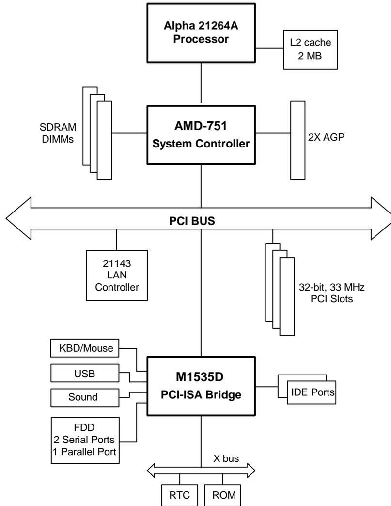
**Figure 1-1 UP1100 Functional Block Diagram**
