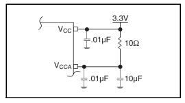
Figure 2. Power Supply Filtering
