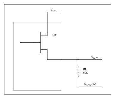
Figure 7. LVPECL Driver Circuit and Termination
