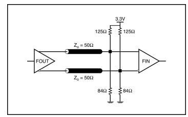
Figure 5B. 3.3V LVPECL Output Termination
