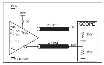
3.3V LVPECL Output Load AC Test Circuit
