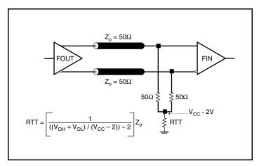
Figure 5A. 3.3V LVPECL Output Termination
