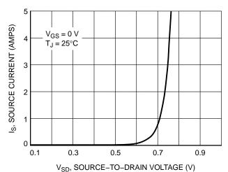
Figure 10. Diode Forward Voltage versus Current
