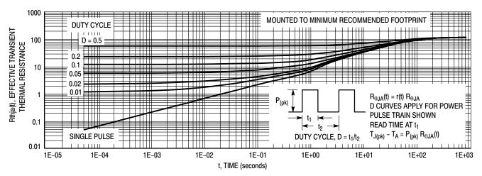
Figure 13. Thermal Response - Various Duty Cycles
