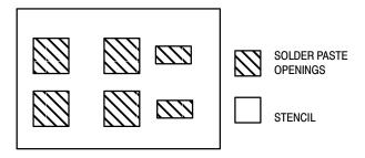
Figure 14. Typical Stencil for DPAK and D<sup>2</sup>PAK Packages
