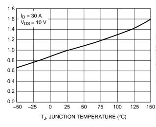
R<sub>DS(on)</sub>, DRAIN-TO-SOURCE RESISTANCE (NORMALIZED)
