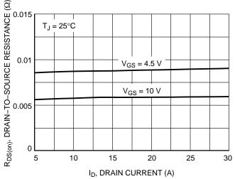
Figure 3. On-Resistance versus Gate-To-Source Voltage
