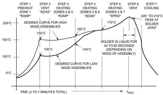
Figure 15. Typical Solder Heating Profile
