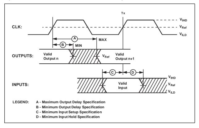
**Figure 9. CLK Timing Measurement Points**
