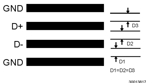
FIGURE 9. Ideal Diode Trace Layout
