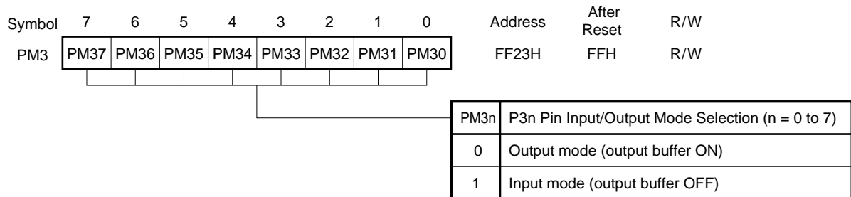
Figure 13-4. Port Mode Register 3 Format
