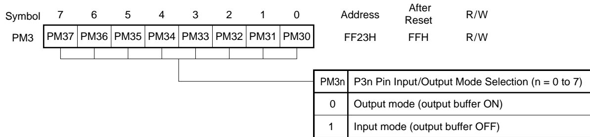
Figure 14-3. Port Mode Register 3 Format
