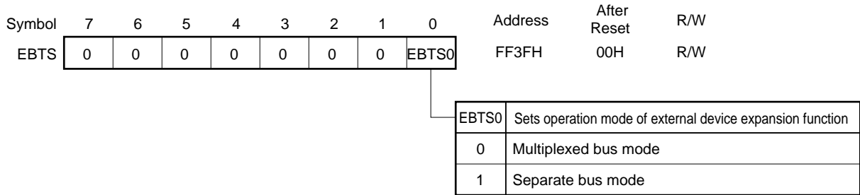
Figure 23-4. External Bus Type Select Register Format
