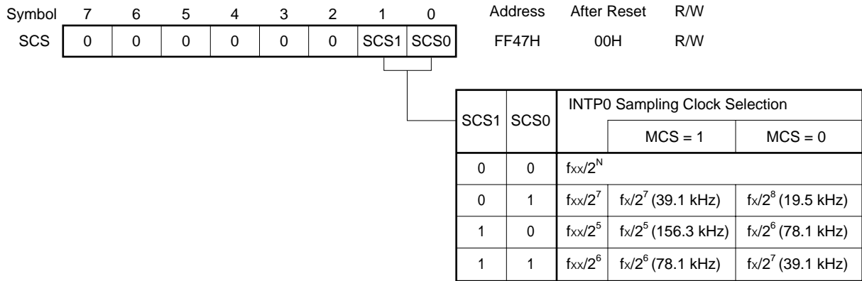
Figure 8-9. Sampling Clock Select Register Format
