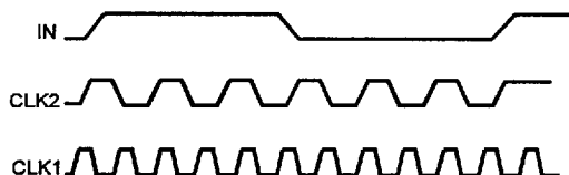
Figure 8: Input and Output Clock Waveforms with CLK2 Connected to FBIN
