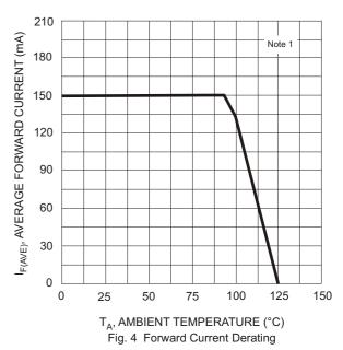
Note 1: Part mounted on FR-4 board with recommended pad layout, which can be found on our website at http://www.diodes.com/datasheets/ap02001.pdf.
